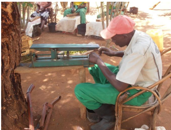
Figure 8: Cracking a nut by use of the cracking device
